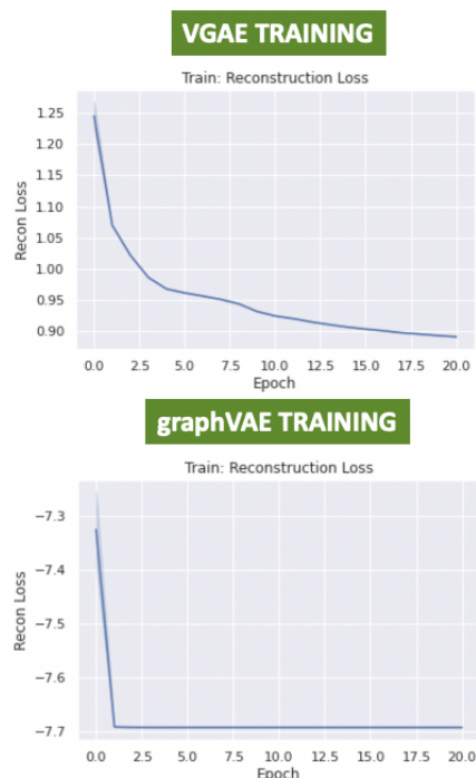
Fig. 7. Training: Reconstruction per Epoch, Experiment 2; 16 Channel, 2 Conv Experiment, VGAE training had learning rate 1e-3, graphVAE training had learning rate 1e-4
