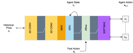
Figure 5. Model-free Policy Gradient (PG) architecture. \rho_{T-t \rightarrow t} \in R^{M \times T} are passed through two 2D-convolution layers, which generate a feature map, which is, in turn, processed by the GRU state manager. The agent state produced is combined (via matrix flattening and vector concatenation) with the past action to estimate action-values q_1, \dots, q_M
