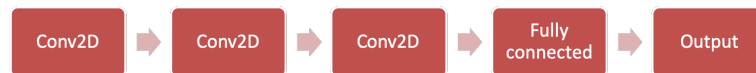
FIG. 2: Illustration of convolutional neural network. The network consists of 3 layers of convolution operations, 1 fully connected layer and 1 output layer.
