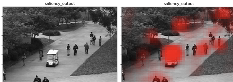
Figure 6: Left: Example image that is predicted to be an anomaly by our model. Right: Heat-map generated by saliency test on the input image. Note that the golf cart is the most heavily colored portion of the frame, indicating that the model correctly labelled this scene as anomalous because of the presence of the golf cart.
