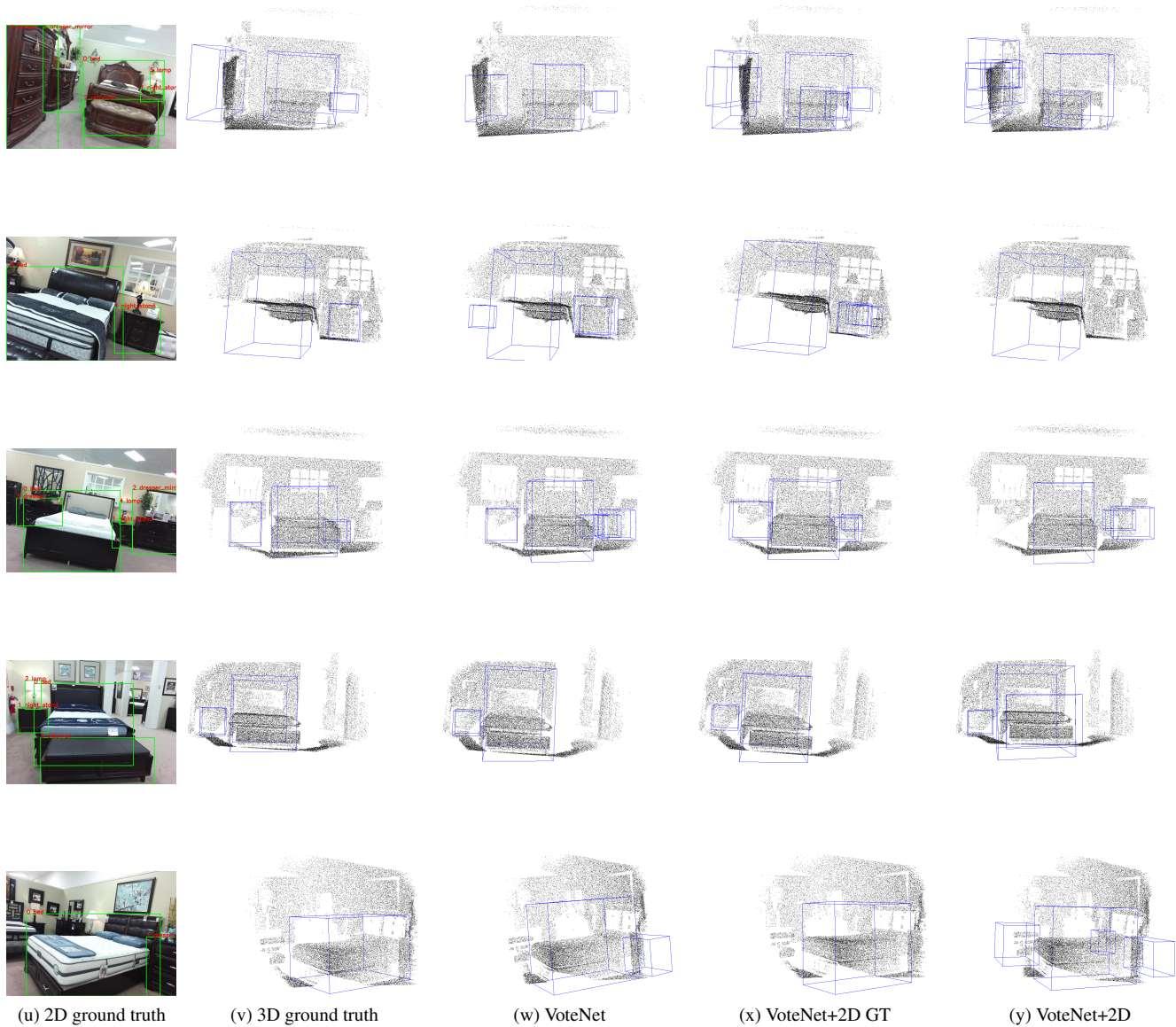
Figure 3: Comparison of result from SUN RGB-D v1 dataset. The first column contains 2D bounding box ground truth from original dataset, and the second column contains 3D bounding box ground truth. Only classes on whitelist are shown in the image. The third column shows result from original VoteNet. The fourth column is from our proposed method using 2D ground truth, and finally the fifth column are produced from our method using RCNN 2D detector.
