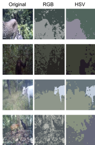
Figure 5: K-means segmentation examples. First column includes frames from sample original videos, the second column includes corresponding output from k-means with RGB features, and the final column includes corresponding output from k-means with HSV features.
