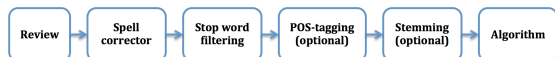
Fig. 3. A pipeline representing the preprocessing of the review data. The last two steps were optional depending on the algorithm used
