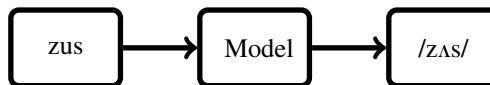
Figure 1. Our model takes Dutch graphemes (e.g. “zus”) as inputs and it outputs a predicted phoneme string.
