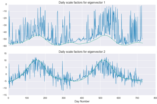
Figure 2: Estimating the clearsky signal by fitting the daily scale factors for the left singular vectors associated with the top two singular values for a single system in the dataset. This process was repeated for all systems and for the summed power signal.
