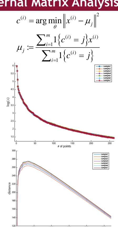
Use sorted eigenvalue from Gaussian kernel matrix versus data points and distance versus data points to determine the number of groups.
