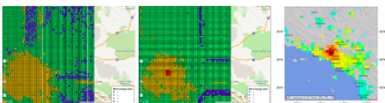
FIG. 9: a) RF BDI, b) SVM BDI, and c) Scaled CDI damage state plots of the Northridge 1994 earthquake
