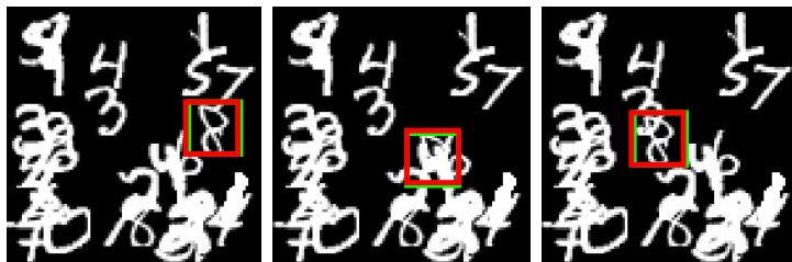
Figure 2: This image sequence depicts the successful tracking of an object following a sinusoidal motion profile through dense clutter (30 objects). (Track Box – Green, True Location – Red)
