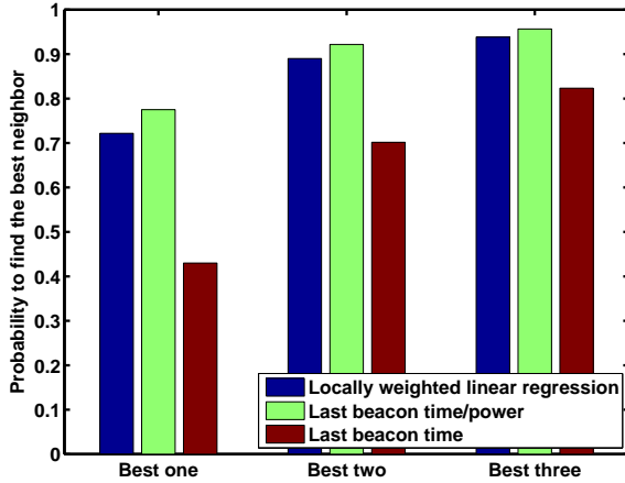
Fig. 2. Probability to find the best neighbor for locally weighted linear regression and naive methods in two-ray ground propagation model
