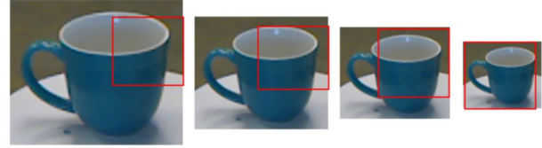
Figure 4. Representation of the image pyramid and sliding window techniques
