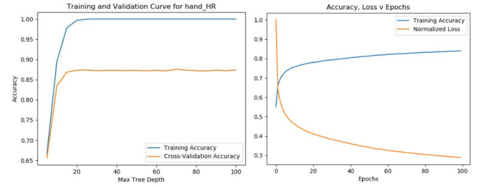
Fig. 4. Left: Training and Validation Curves for Limited Feature-set using Ordinary Decision Trees. Right: Training loss and accuracy for the Multilayer Perceptron neural net when trained on the reduced feature-set.
