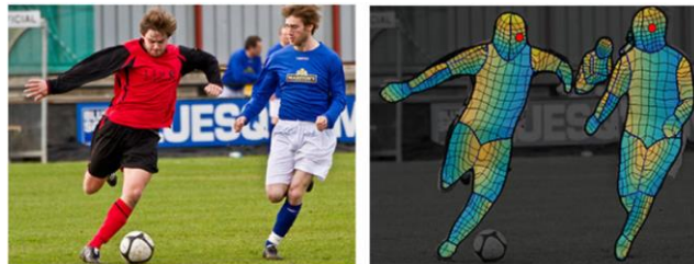
Figure 1: A sample RGB image (left) processed by DensePose (right). Each pixel is assigned to a corresponding point on a human skin mesh [6].
