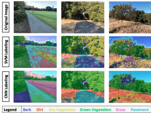
Figure 6: Multi-terrain images categorized using the sliding window algorithm paired with the SVM and CNN classifiers.
