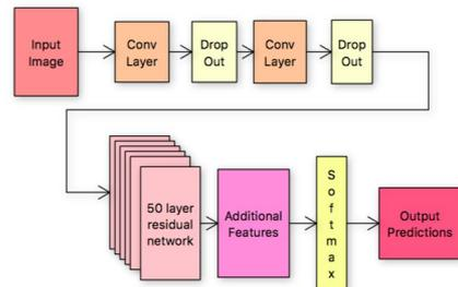
Figure: neural net architecture combining residual network with additional features to output softmax prediction.
