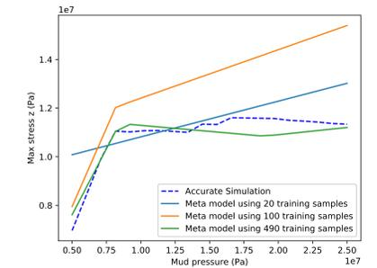
Figure 7: Prediction of Max. stress Z as a function of the mud pressure for Max.degree = 2 and Penalty = 3.0
