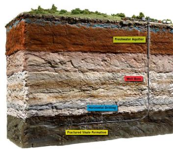
Figure 2: Horizontal wells for hydraulic fracturing
