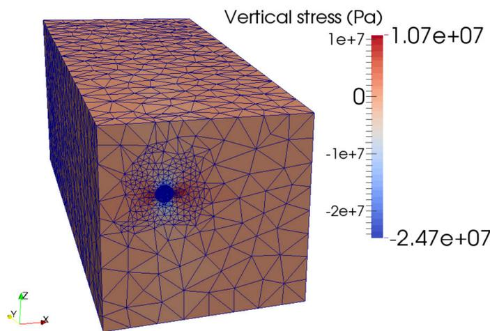
Figure 3: Finite element simulation result (vertical stress contour)
