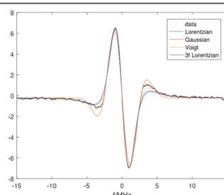
Voigt model, a convolution of Lorentzian and gaussian functions, gave the best fit to spectral data.
