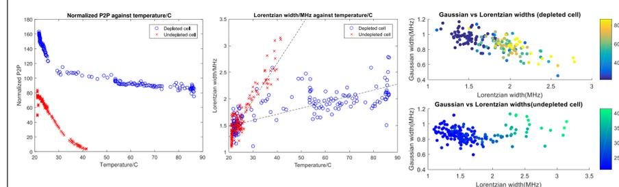
Weighted linear regression was used to fit temperature dependence of Lorentzian width. The weight was proportional to  $(\text{peak-to-peak})^2$  to prioritize stronger signals obtained at lower temperatures.
