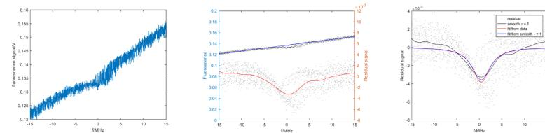
Linear baseline and Lorentzian curve fitting were performed on fluorescence data. Data noise resulted in 50 times higher error than fitting the 3<sup>rd</sup> derivative spectra directly.
