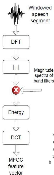
The features vector selected are the Mel-frequency Cepstrum coefficients (MFCC). It transforms the frequencies to a mel scale, which has two set of filters: one spaced linearly for frequencies below 1000 Hz and one spaced logarithmically above 1000 Hz. we extract 20 MFCC features for each time frames that lasted 93 ms and spaced 23 ms apart.
