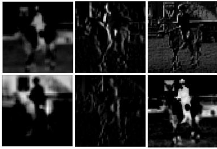
Figure 6 Layer 1 outputs, same column is from the same model. From left to right: K=15 K=11, K=7
