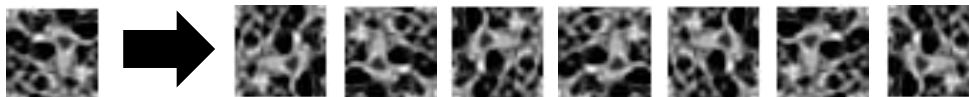
Figure 2. Example of Rigid Transformations. The original image patch was rotated and reflected in order to create additional images per texture class.
