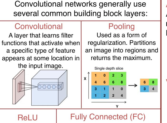
Increases the nonlinear properties of the decision function using the activation function f(x) = max(0, x)
