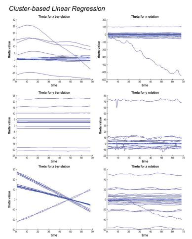
The most effective method was a combination of the previous approaches. We used linear regression on each cluster to generate a set of thetas for each class of joint. The linear regression uses the input position of the joint in order to output the set of time-varying translations and rotations.
