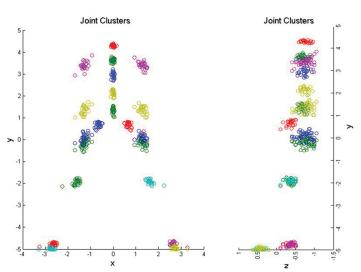
The sample data holds many joints of different types, which lends itself naturally to a clustering algorithm. Joints are clustered based on the set of input features described above. A test joint is then assigned to a cluster, and the output animation is the average of the animation curves of all training points in the cluster.
