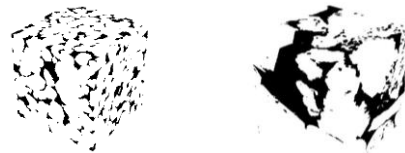
Figure 1: 3-D images of Fontainebleau sandstone (left) and Berea sandstone (right). The white color represents grains and black color represent pore space.
