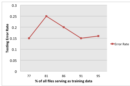
Figure 6. Error rate of different percentage of total files serving as training data
