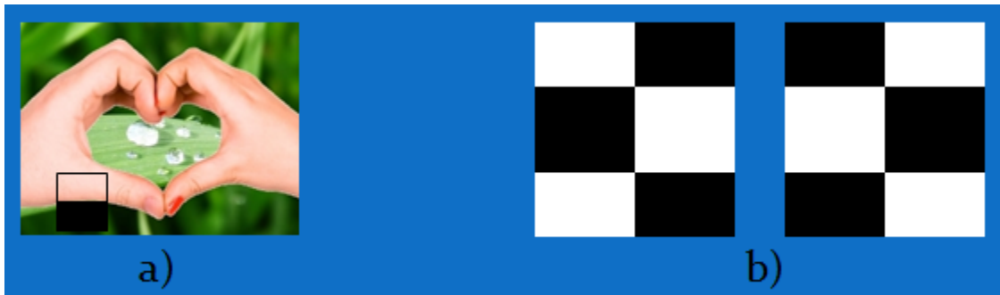
Figure 4. a) Find edges using edge Haar-like features. b) C-shape Haar-like features.
