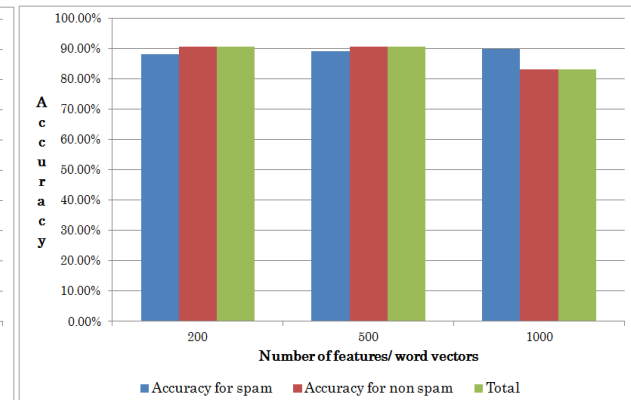
Fig 4. Plot showing accuracy vs. number of features using Chi-2 feature selection and Gaussian kernel
