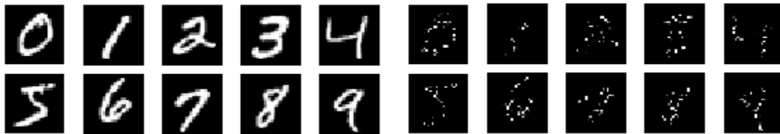
Figure 2 – (left) example digits from the MNIST dataset, (right) the same digits with 85% of the pixels removed, simulating sparse data. Note that some digits remain human-recognizable, but others do not.
