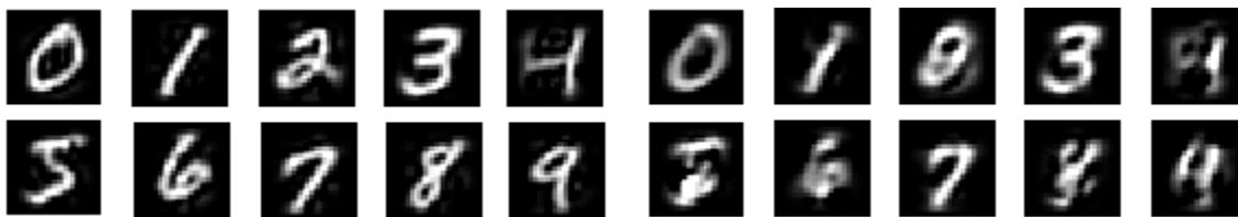
Figure 4 – (left) collaborative filtering with k=60 with no pixel corruption, (right) collaborative filtering with k=20 and 85% pixel corruption. Note that several digits become much more human-recognizable (compare with Figure 2).
