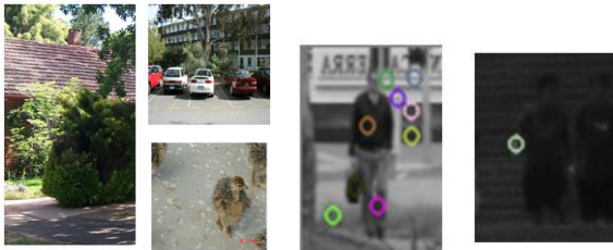
Figure 11 [Left]: Where's Waldo? SURF labeled these images as human. [Right]: Low keypoint images are often misclassified by FREAK and BRISK.
