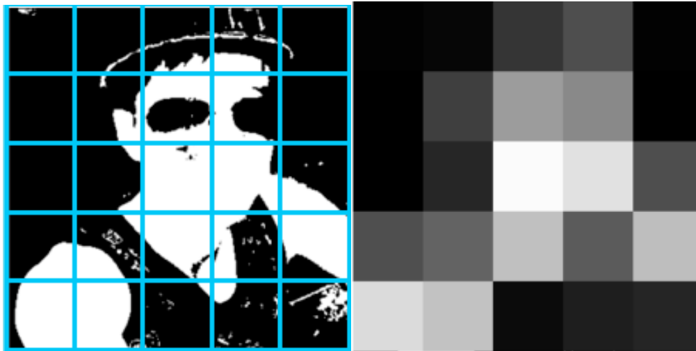
Figure 3. Partition a binary image into 5x5 blocks Figure 4. The visualization of the result of regionization
