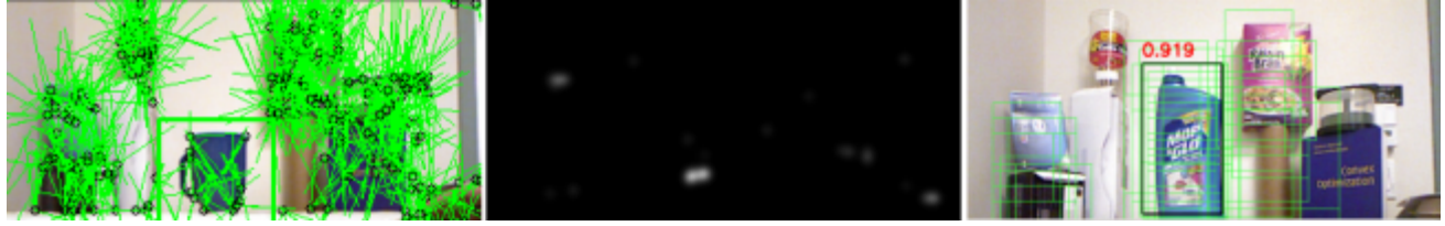
Figure 2. Left: Visualization of Hough voting method. Every black circle is a weakly-detected part, and green lines indicate votes. The green lines meeting at the center of the tea cup give rise to a noticeable peak in the response map for that object ( Center ). Right: Visualization of the root filter template matching. Proposed locations are shown in green and filtered further. The black rectangle is a true positive match obtained from subsequent filtering.
