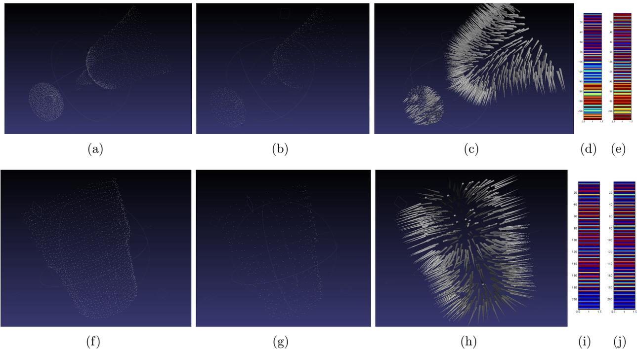
Figure 1: Point Clouds Normals Computation and Histograms Generation : First is our original point cloud, Second is the downsampled point cloud followed by the display of the computed normals. Two Histograms are shown with colder colors corresponding to lower values. These histograms are computed for a discretization of each angle into 6 bins. Their size is  $6 \times 6 = 216$ .
