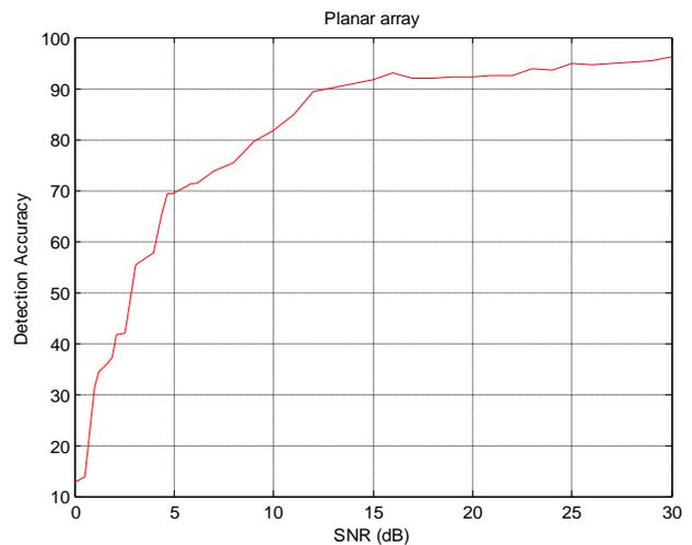
Accuracy vs SNR for a 5\*5 planar array
