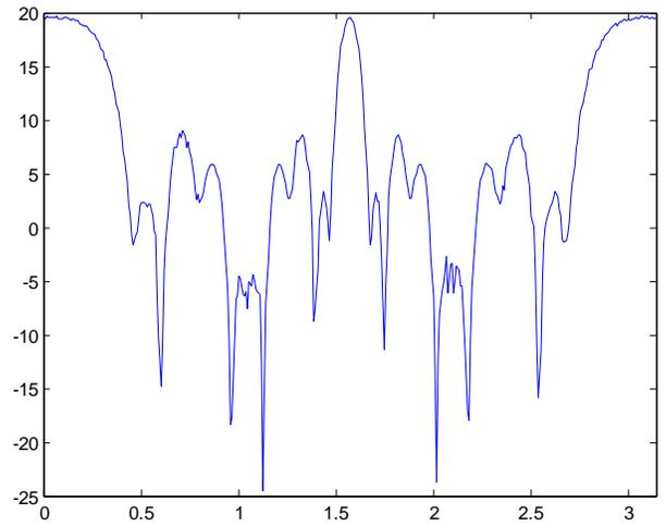
Distorted pattern of a faulty antenna
