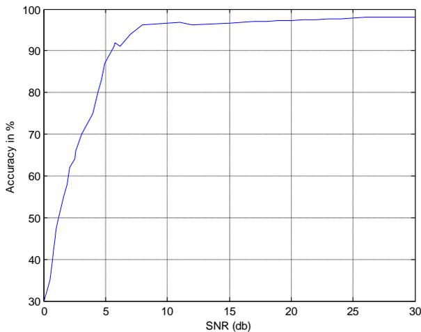
Accuracy vs SNR for a 11 element linear array
