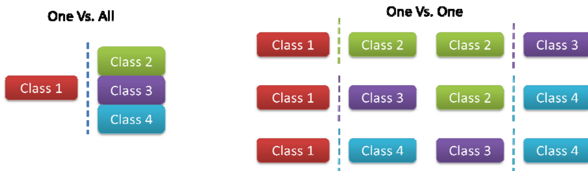
Figure 4: Brief comparison of the two multi-class SVM approaches. Note that, in this example, the One Vs All approach will require three more SVM comparisons
