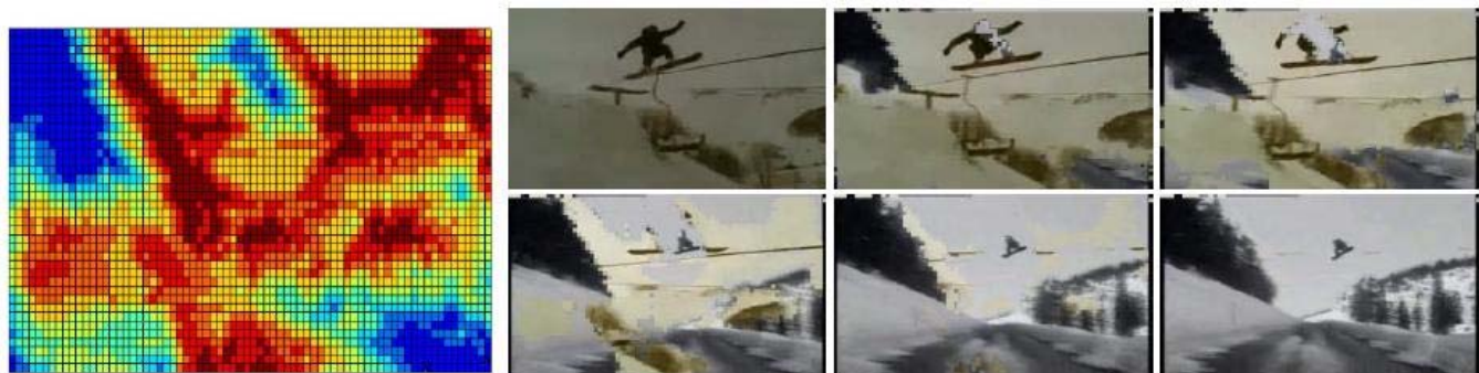
Figure 5: Joining videos: Some frames from the transition of two videos. We can observe that the videos have been joined at a position of similar content, and the snowboarders from the two videos have been matched. Figure also shows the seam along which the videos are joined.
