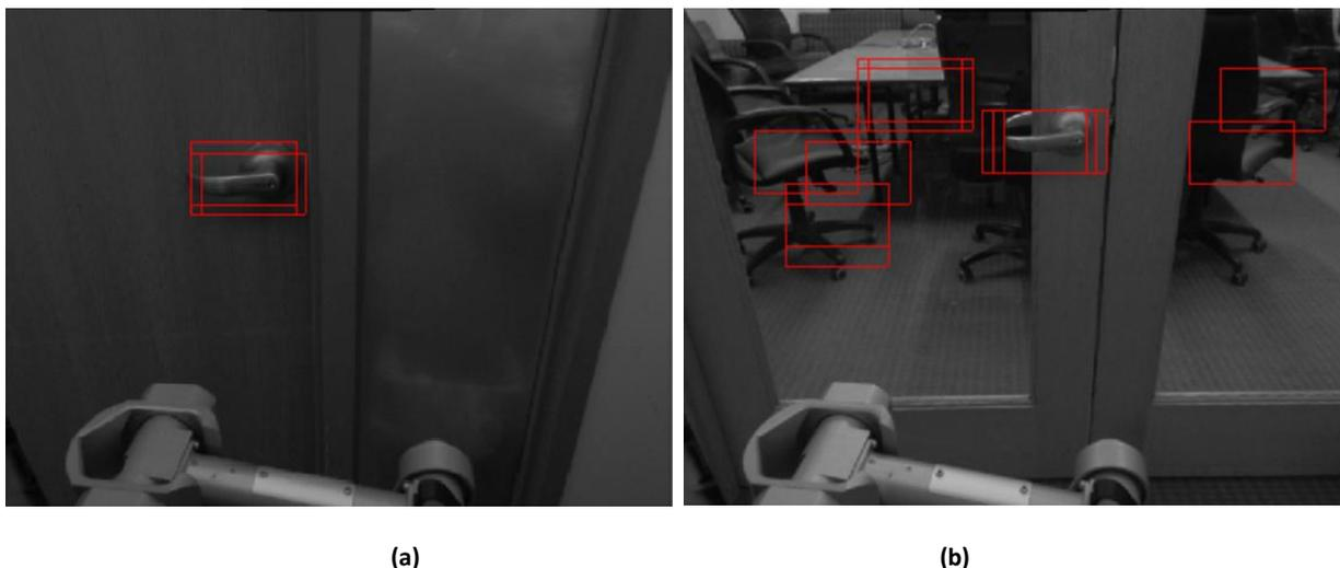
Figure 2 – Sliding Window results for (a) opaque and (b) glass doors
