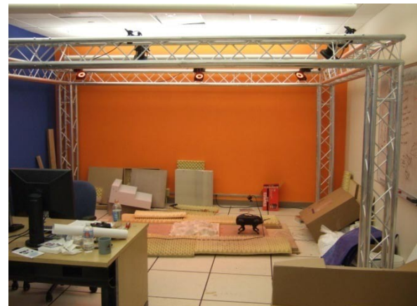
Figure 2. Motion Capture System, built by Vicon MX system
