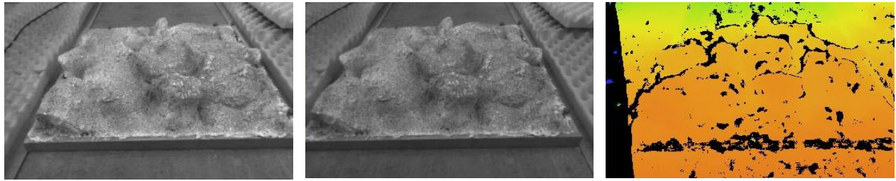
Figure 4. Left, Right Images and Depth Map from a stereo vision, made by Tzyx Inc.
