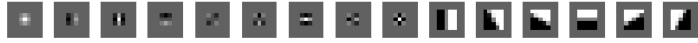
Figure 5: The filters used for computing texture variations and gradients. The first 9 are Laws' masks, followed by the oriented edge filters.
