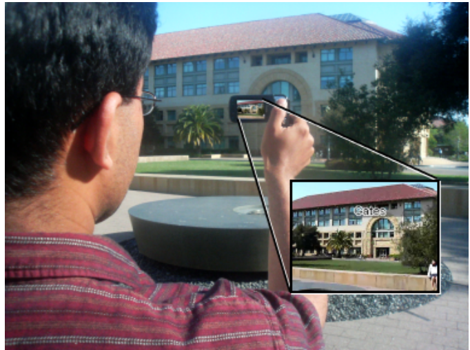
Fig. 1. A snapshot of the outdoors augmented reality system being used. The system augments the viewfinder with information about the objects it recognizes in the image taken with a phone camera.
