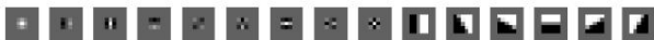
Figure 2: Image Texture Features. The first nine images are Laws mask filters, followed by the texture gradient filters.
