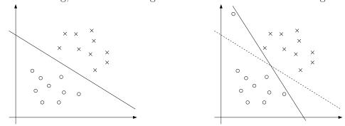
To make the algorithm work for non-linearly separable datasets as well as be less sensitive to outliers, we reformulate our optimization (using  $\ell_1$
