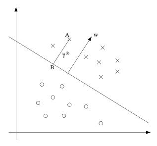
The decision boundary corresponding to (w, b) is shown, along with the vector w. Note that w is orthogonal (at 90°) to the separating hyperplane. (You should convince yourself that this must be the case.) Consider the point at A, which represents the input  $x^{(i)}$  of some training example with
