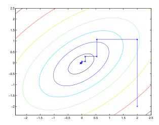
The ellipses in the figure are the contours of a quadratic function that we want to optimize. Coordinate ascent was initialized at (2, -2), and also plotted in the figure is the path that it took on its way to the global maximum. Notice that on each step, coordinate ascent takes a step that's parallel to one of the axes, since only one variable is being optimized at a time.
