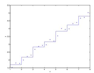
This piecewise constant representation just isn't a good representation for many smooth functions. It results in little smoothing over the inputs, and no generalization over the different grid cells. Using this sort of representation, we would also need a very fine discretization (very small grid cells) to get a good approximation.
